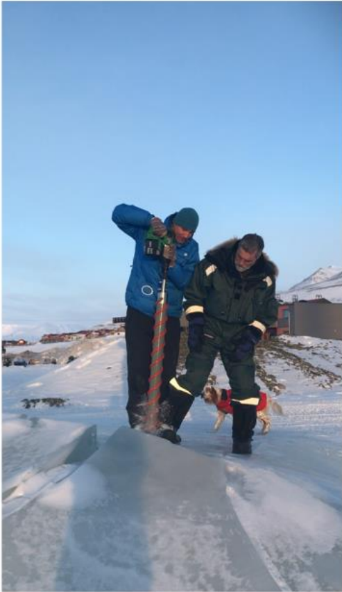
Figure S1.a2-4. Snapshot from Video S1.a2-1 (Sinitsyn, 2023a). Drilling through small, cracked "mound" icing at Longyearlva behind Elvesletta Nord (18.04.2017, location a2 in Table S1). Video: © Anatoly Sinitsyn.
