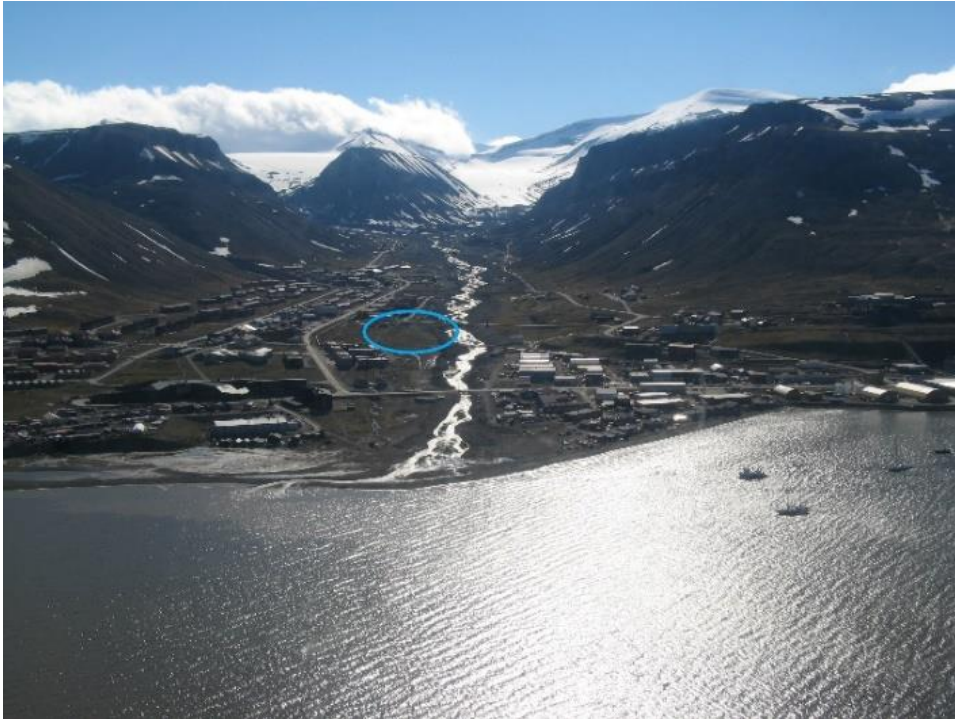
Figure S1.a10-1. Longyearrelva channelled into one large riverbed equipped with rock- protection of riverbanks against erosion (2017). Blue circle depicts approximate location of Elvesletta. Photo: © A. Skoglund / Norwegian Polar Institute.
