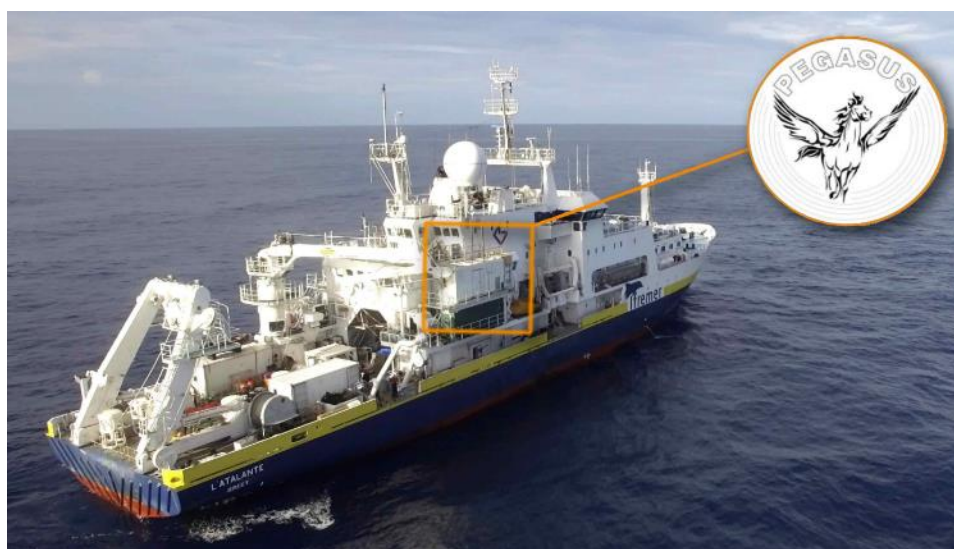
Figure 37. View of the PEGASUS container laboratory for the monitoring of the composition/physical characterisation of the lower atmosphere: this was continuously performed during TONGA.
