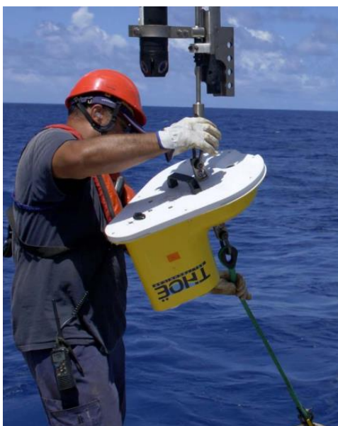
Figure 33. A THOE instrument installed on the TONGA fixed mooring.
