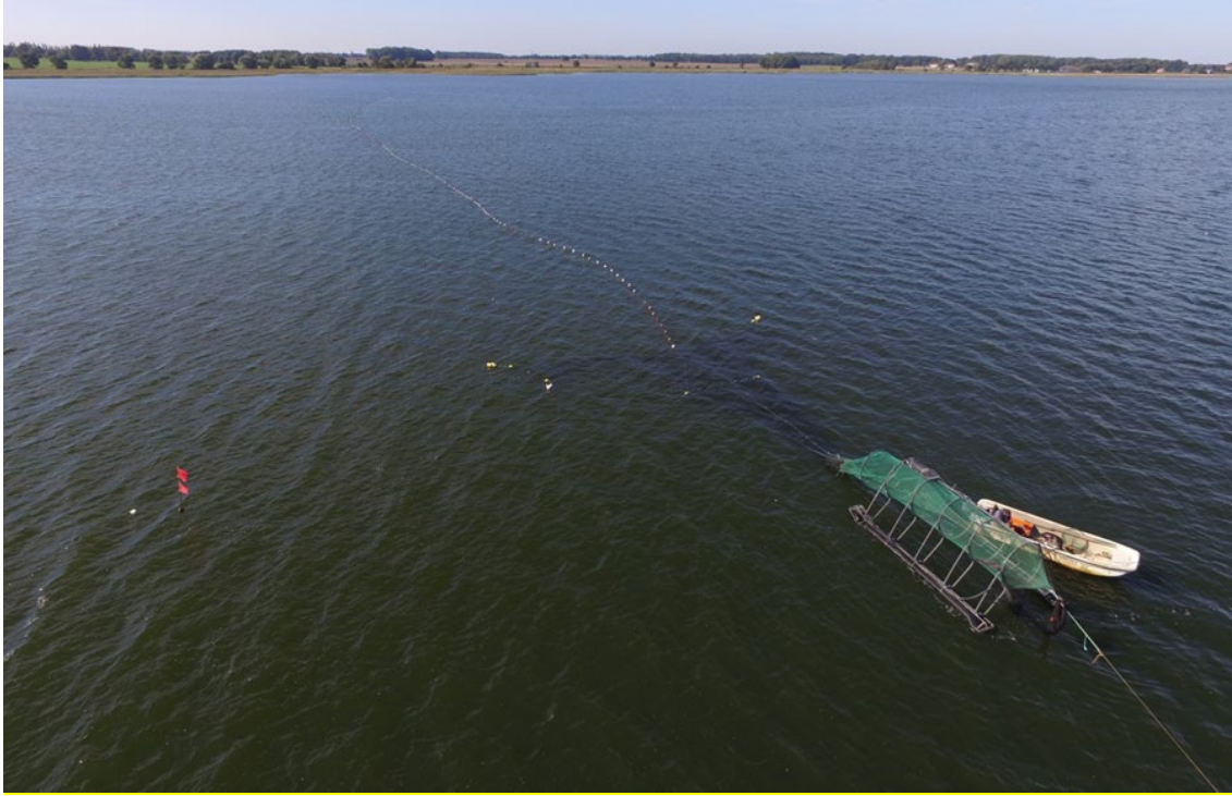
Figure 7.31: Pontoon trap in German waters (water depth at position of pontoon trap is approx. 3 m). Picture shows the original design. Several improvements were tested.
