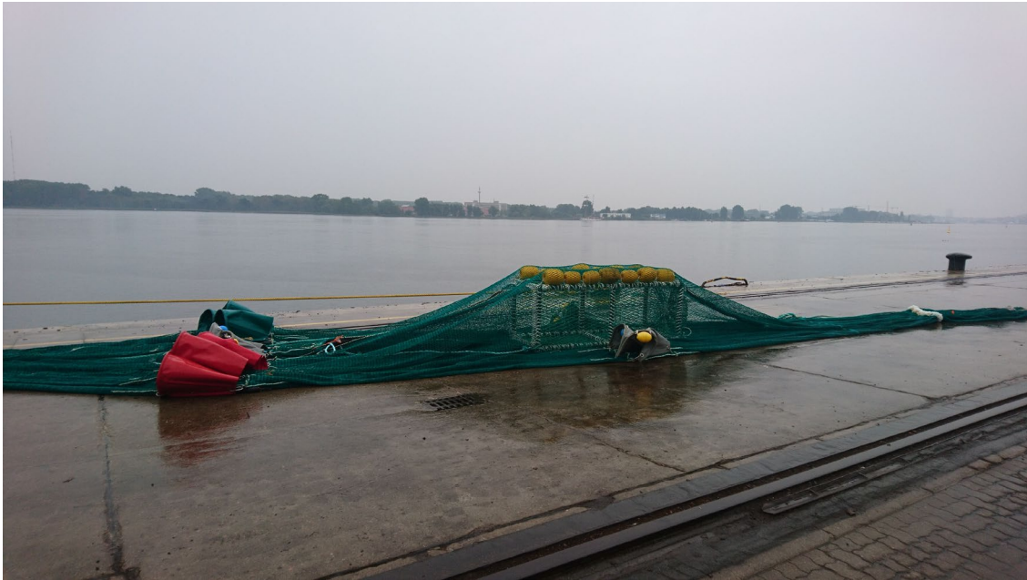
Figure 7.22: Experimental codend with fixed meshes inside the cover codend.
