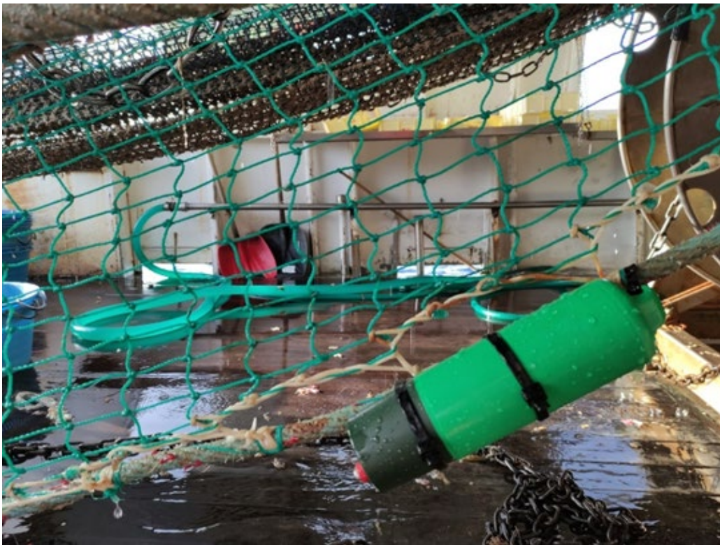
Figure 7.45: Project DELFI; Dolphin deterrent device
