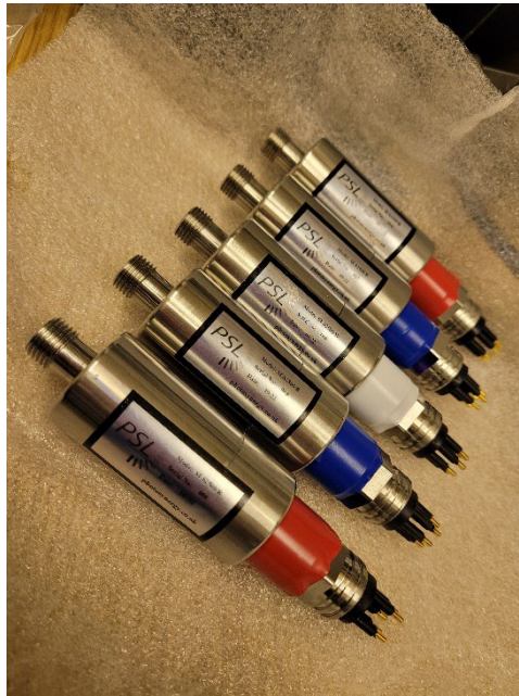
Figure 7.61: Photosynergy Limited LED light pods to illuminate fibre optic (FO) cables
