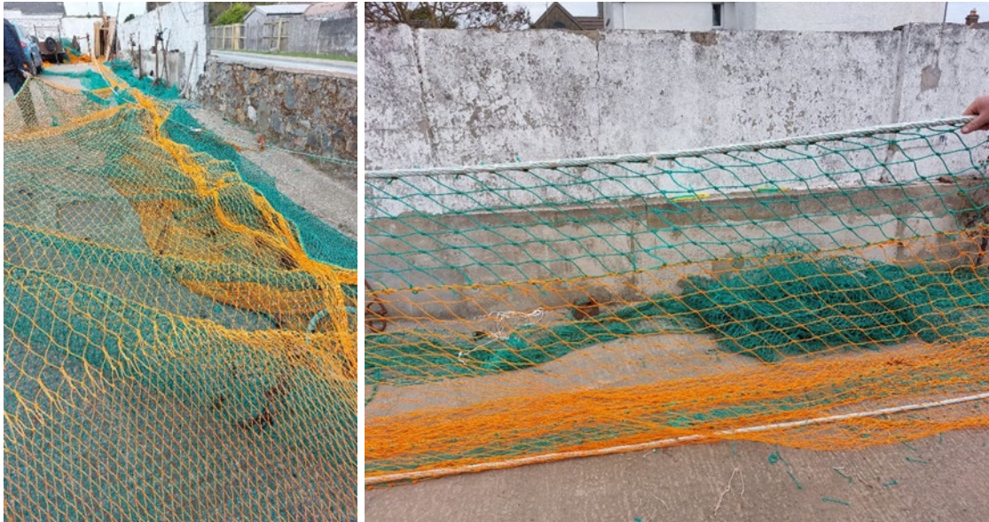
Figure 7.69: Coverless nephrops trawl with 160mm diamond mesh netting fitted into the top sheet (left) and wings (right). The original 80mm netting in the top sheets remained in the first part of the tapered section to prevent loss of nephrops.
