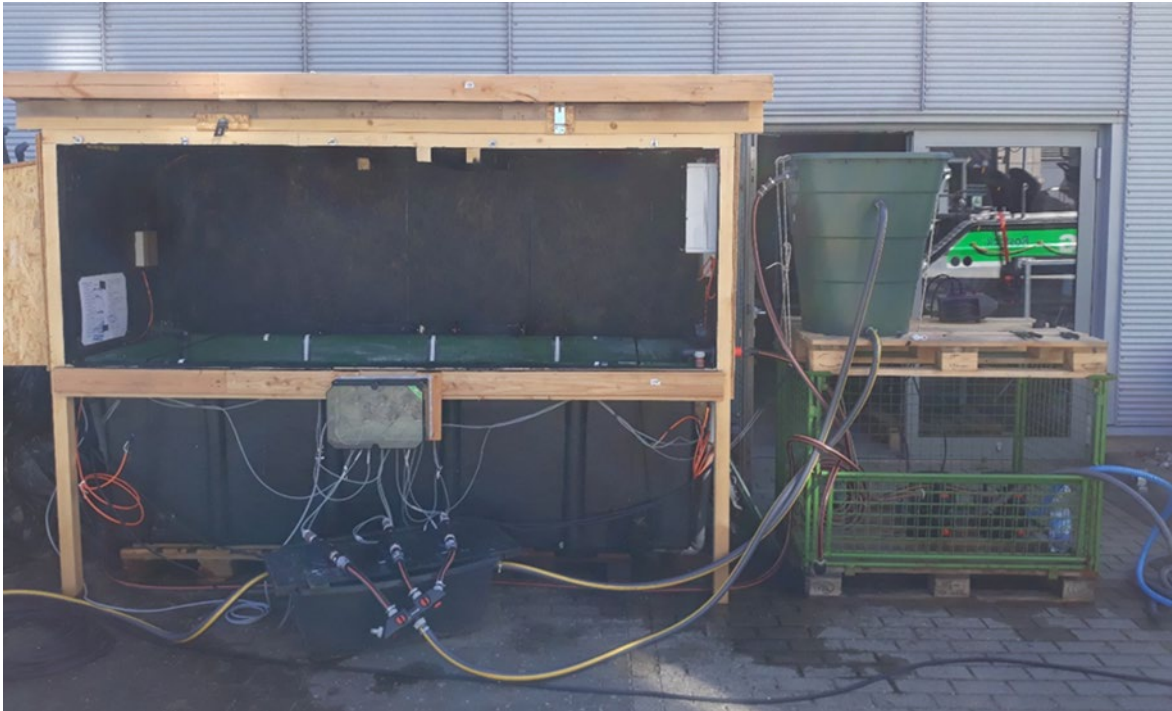
Figure 7.29: Bait-experiments: experimental setup for automatic bait choice experiments. The inflow of bait water is realized by a number of pumps which are automatically computer-controlled. The behaviour of fish is automatically recorded using an IR-camera system
