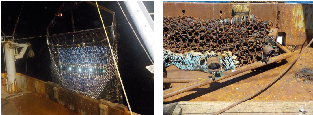
Figure 7.81: (Left) Pisces LED lights located in the middle of the twine top with the square mesh escape panel in constant white light. (Right) location of Pisces LED lights welded to the bale bar of the scallop dredge.
