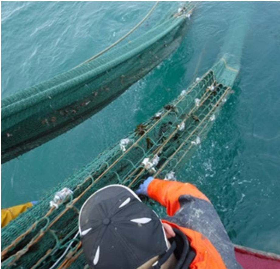
Figure 7.64: Lights attached to square mesh panel fitted into nephrops trawl
