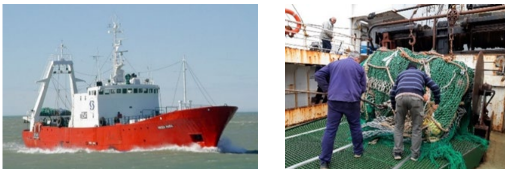
Figure 7.4: Stern trawler “Virgen María” and trawl net on net drum.
