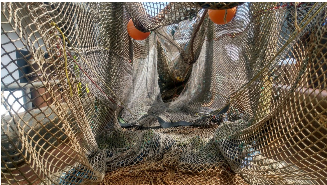
Figure 7.82: ActSel selection panel (lighter grey, smaller mesh) and kite installed in a trawl.
