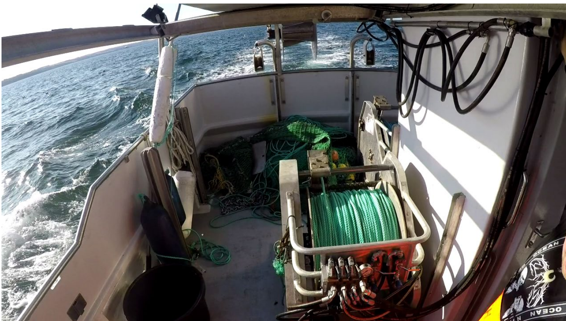
Figure 7.33: Mini seine system installed onboard the Danish fishing vessel being involved in previous work with it.
