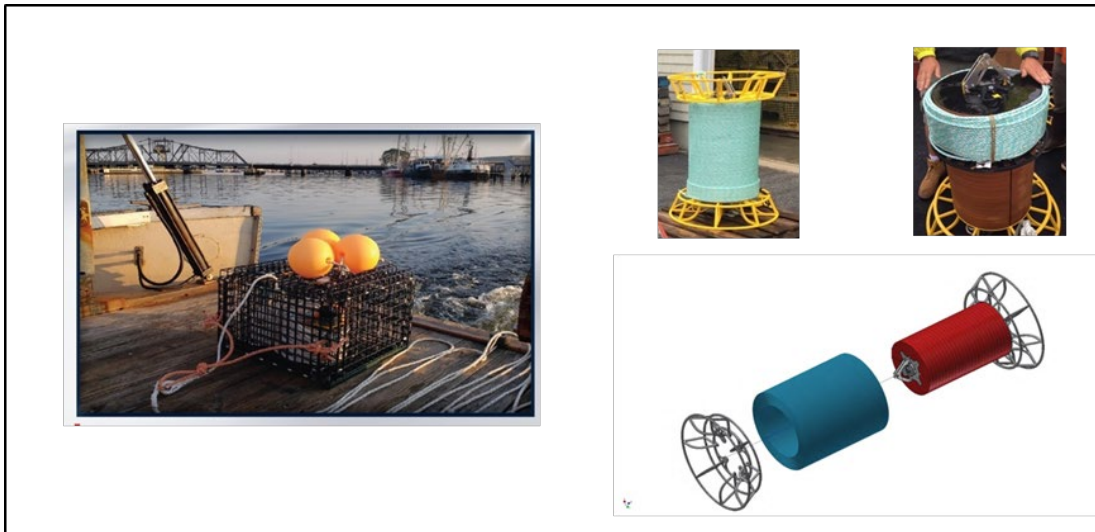
Figure 7.83: The two ropeless systems tested during the field trial. Left: the Edgetech trap in which the vertical line is coiled inside an empty trap before hauling. Upper right: the flotation spool with the line coiled about and showing placement of a “coil pack” over an empty spool; at bottom is an engineering diagram of the spool. An acoustic release is placed in the center of the spool.
