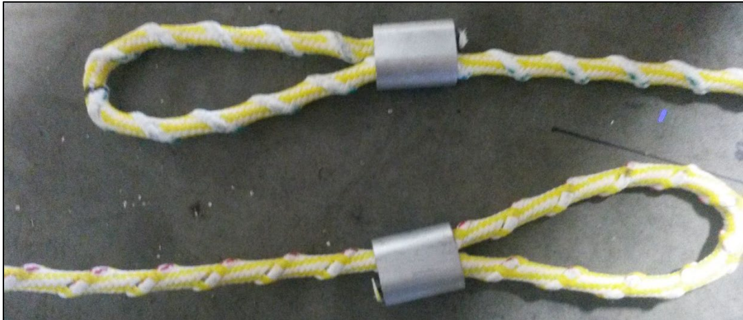
Figure 7.75: Helix twine with markings delineating the direction of coils, clockwise (red; bot-tom) and counterclockwise (green; top).
