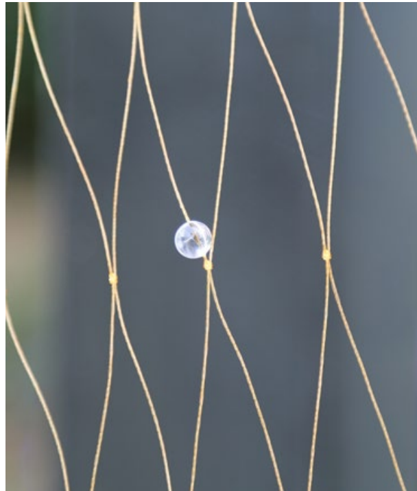
Figure 7.26: Gillnet with Acrylic-pearl (diameter: 8 mm)
