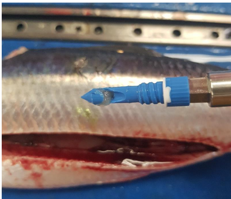
Figure 6. The extracted GST showing the tissue sample retained within the sample collection window.
