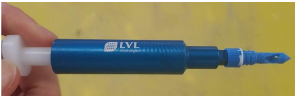
Figure 3. The GST in place on the manual decapper tool, which functions as a handle.
