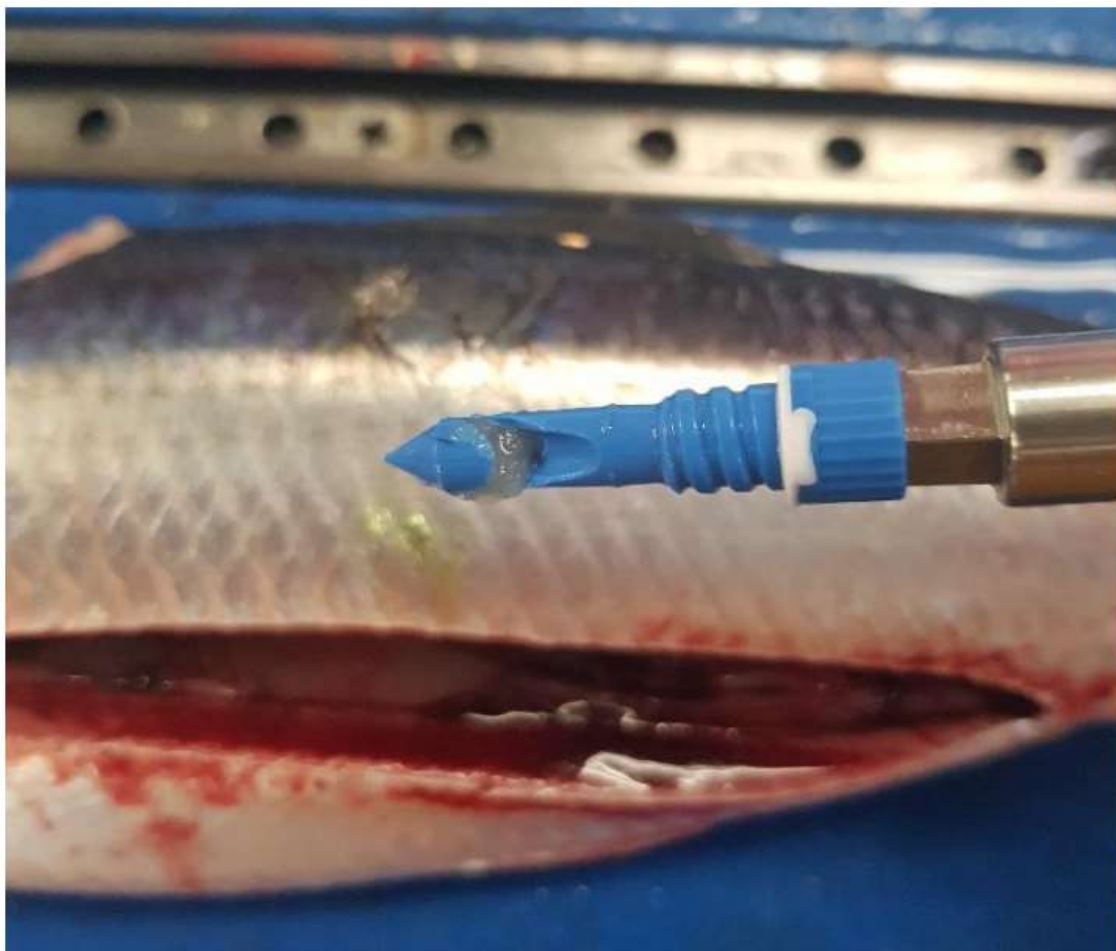
Figure 3.5.1. An extracted Genetic Sampling Tool (GST) showing the tissue sample retained within the sample collection window. See Annex 6 for further illustration and operating procedure.
