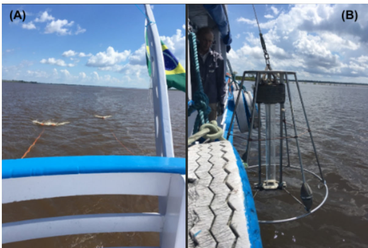
Figura 1. (A) Seismic equipment in acquisition and (B) Coring equipment being deployed, both from Samara Lopes XII vessel.
