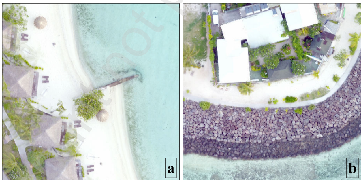
Figure 7: Examples of the two main types of shoreline protective structures found on the Bora Bora study site. Perpendicular (a) and parallel (b) to the water line.
