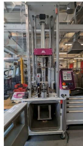
Fig. 2. (A) 16 mm diameter hemispherical impactor, (B) 12.7 mm diameter conical impactor and (C) Instron CEAST9350 drop weight impact tower.
