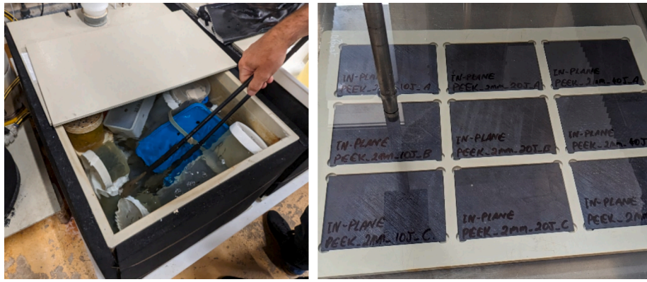
Fig. 3. (a) Hydrothermal seawater ageing tank showing specimen removal for weighing and (b) Ultrasonic C-scanning setup showing vertical probe with transducer.
