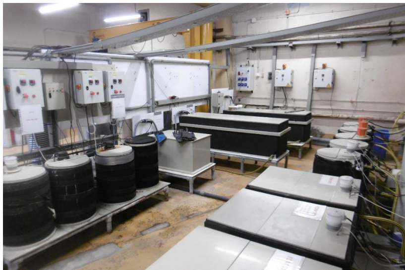
Figure 1. Seawater aging facility, low pressure tanks
