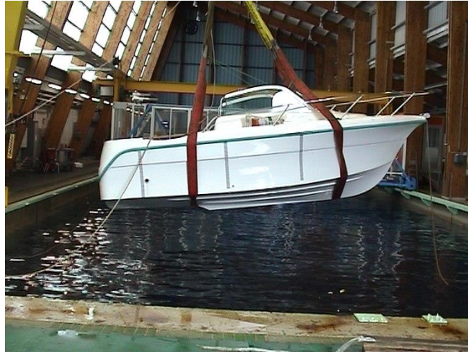
Figure 5. Instrumented boat drop in test tank [36]
