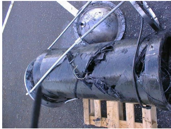
Figure 9. (Left) 1000 bar pressure vessel, (Right) Strain gauged cylinder, (Lower) Composite cylinder after implosion testing.
