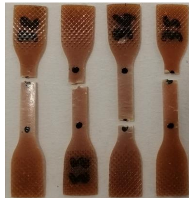
Figure 6. Tensile tests on bulk adhesive specimens.
