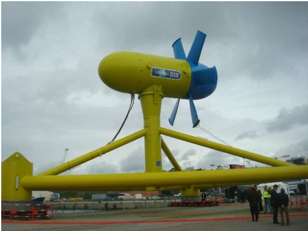
Figure 22. Tidal Turbine developed by Sabella, Quimper, France, with 5-meter long carbon/epoxy blades [188]
