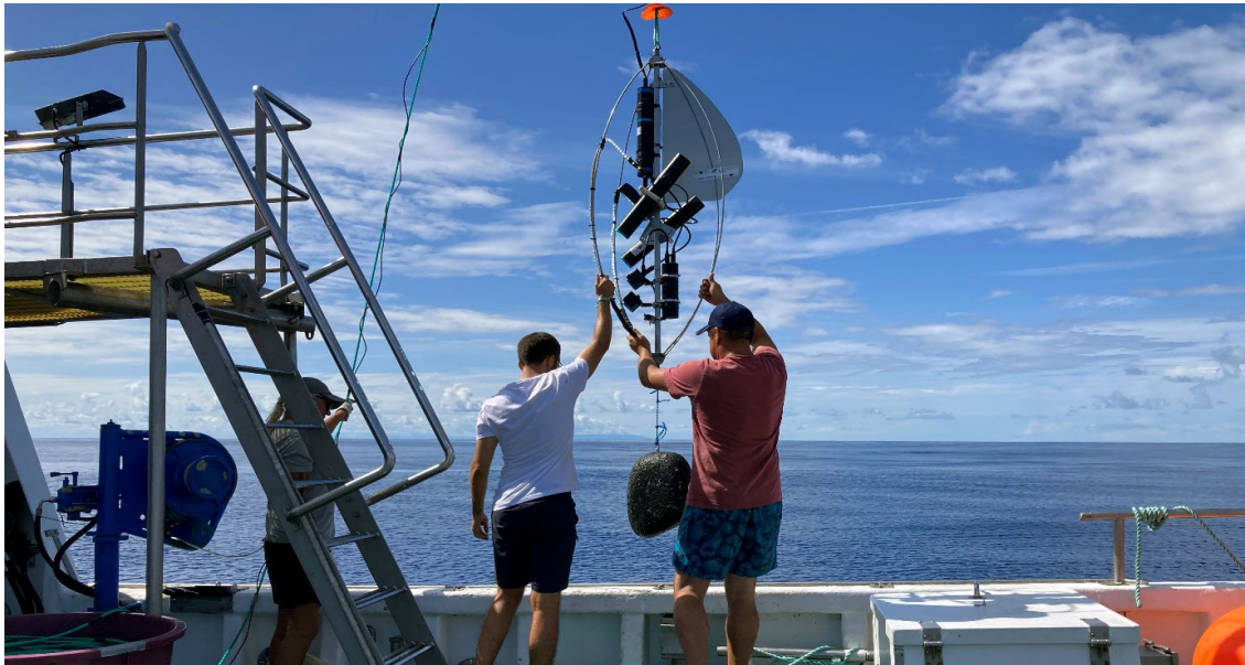
Figure A4.4. Members of the ADSR group deploying the Azor drift-cam from the side of the N/I Arquipélago to explore deep-sea areas shallower than 1000 m depth in the Azores.
