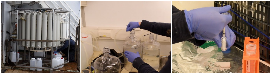
Figure A4.7. Collection and processing of water samples to extract eDNA for biodiversity assessments during one of the cruises led by ADSR.
