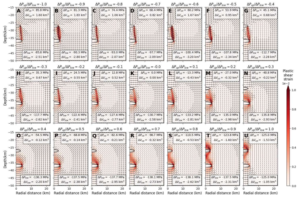
Figure S6: Plastic shear strain generated by different \Delta P_{up}/\Delta P_{low} ratios, for two sill-like reservoirs. Each subplot represents the final stage of a run shown as dots in Figure S7. Subplots A, K and U correspond to Figures S7B, C and D, respectively. Reservoir separations (height between the roof of the lower reservoir and the base of the upper reservoir) are identical to Figure S4.
