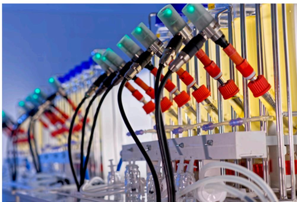
Figure 13. Culture of four strains of Skeletonema marinoi using a phenotyping bench specially designed to grow microalgae under highly homogeneous conditions of temperature, pH and light. Four non-axenic Skm strains were grown in 400 mL photobioreactors in batch mode in triplicate independent assays. Culture conditions consisted of 35‰ salinity sterile seawater enriched by Walne (“Conway”) medium and silica, temperature and pH were regulated at 20 °C and 8.00, respectively, and a continuous white light irradiance was set at 200 \mu\text{mol}\cdot\text{m}^{-2}\cdot\text{s}^{-1} . Copyright: IFREMER. O. Dugornay.
