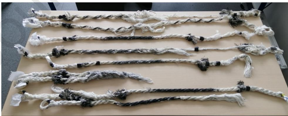
Figure 9 - 4T sub-rope samples after fatigue failure obtained during the MONAMOOR project
