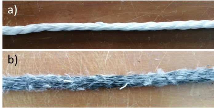
*Figure 11 - Image of the samples analysed with X-ray tomography. a) Virgin sample. b) Sample after fatigue testing and failure in the eye-splice*
