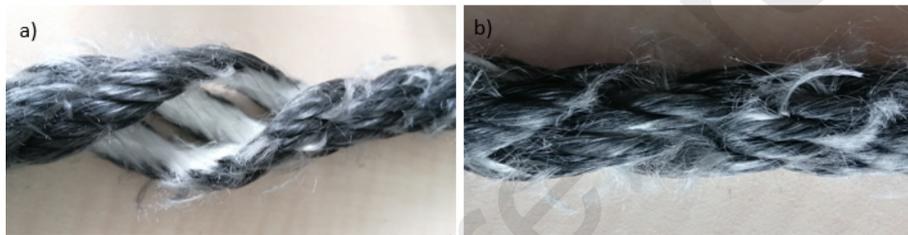
Figure 10 - Damaged 4T sub-rope after fatigue testing
