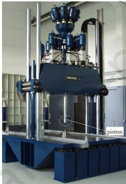
Figure 2 - Servotest hydraulic machine used for testing
