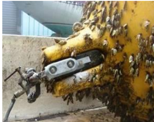
Photo 10: Anode on a 600 liters float.
