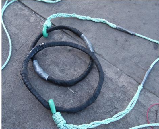
Photo 21: Rings for sandbags anchor.
