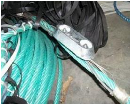
Photo 9: Anode on a combination cable.
