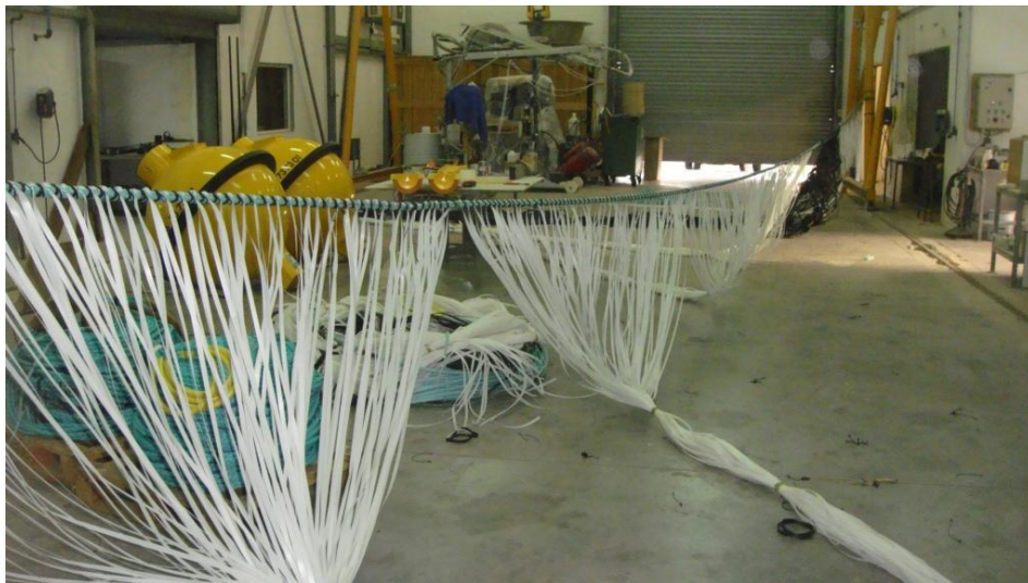
Photo 13: Aggregators in polypropylene strap bands.
