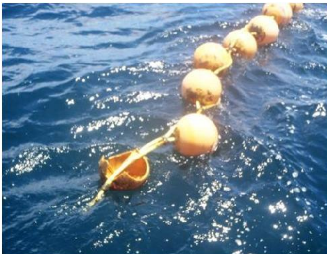
Photo 4: Broken float on a MAGDELESA FAD.
