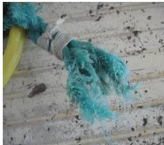
Photo 12: Aspect of a rupture near a kink.
