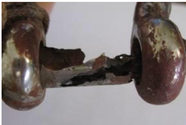
Photo 7: Electrolysis on a stainless steel shackle.
