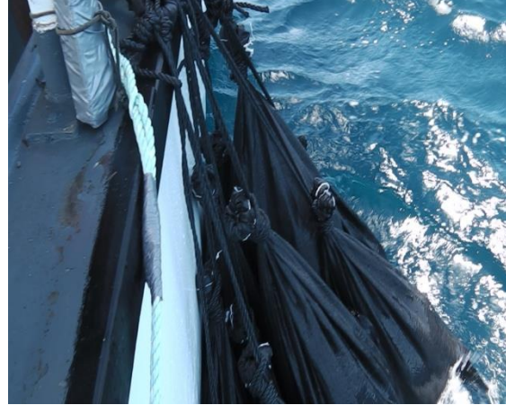
Photo 22: Sandbags anchor alongside the boat.
