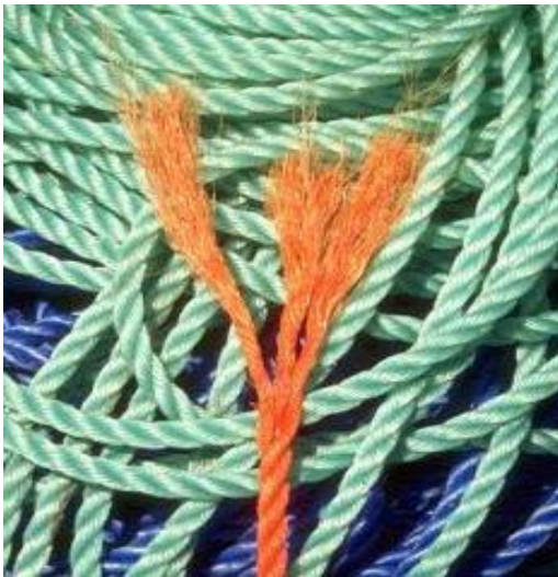
Photo 2: Rupture after excessive tension.
