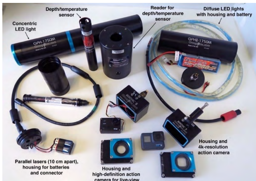
Figure 4. Electronic components used in the Azor drift-cam. All components are mounted on the metallic structure with the exception of the reader for the depth/temperature sensor, which is kept on board to download the collected data after the dives.
