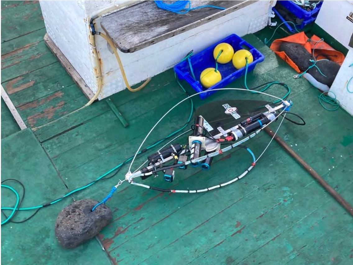
Figure 1. Image of the Azor drift-cam on the deck of the vessel N/I Arquipélago ready to be deployed to obtain images of the deep sea.
