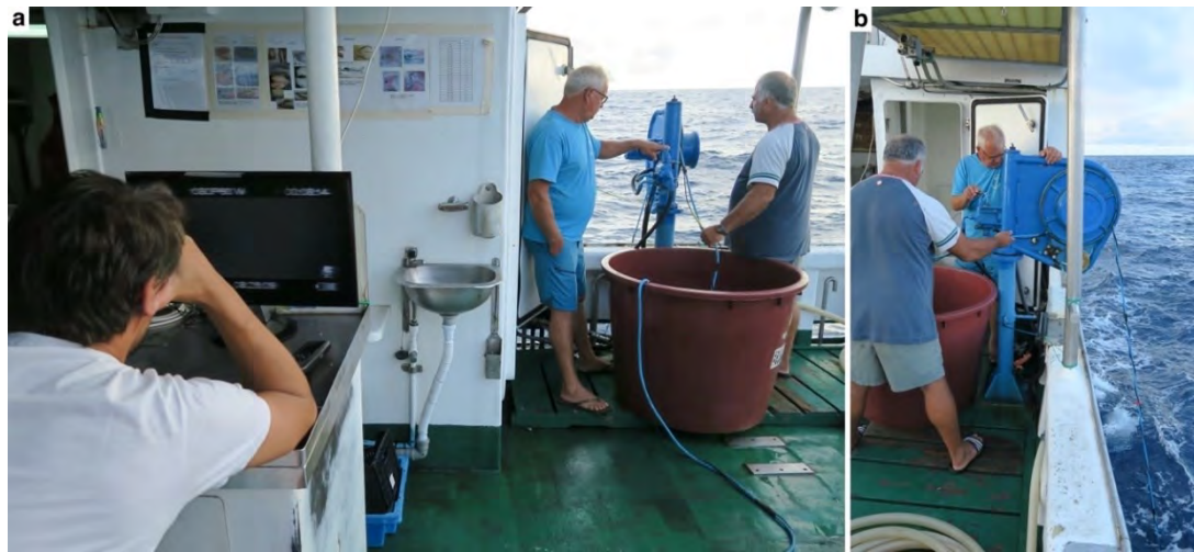
Figure 10. (a) Two members of the Azores deep-sea research group setting up the cameras and batteries of the Azor drift-cam prior to its deployment. (b–c) Deployment of the Azor drift-cam from the side of the vessel using a crane to lift the system.
