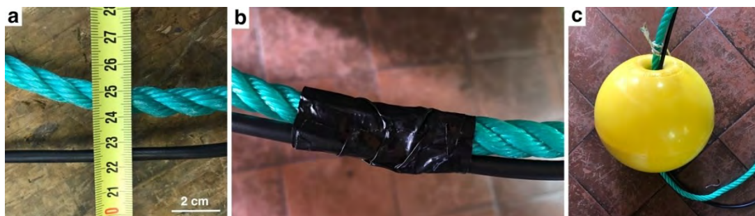
Figure 6. The umbilical. (a) Image of the polypropylene rope (green) and electrical cable (black) used to control the Azor drift-cam and get the video feed to the surface when underwater. (b) Attachment of the rope and the umbilical every meter or so using duct tape. (c) One of the deep-sea floats employed to always keep the drift-cam in an upright position. A thin cord is used to keep the floats in a fixed position on the rope.
