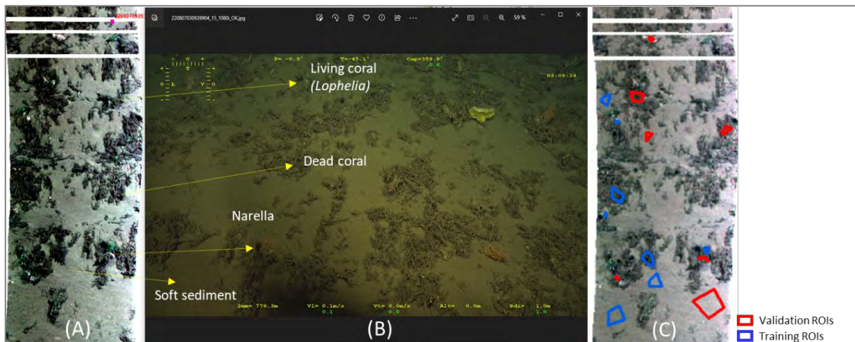
Figure 42. UHI RGB visualisation (A), RGB image from video recorded simultaneously (B), and regions of interest (ROIs) created for training and validating UHI image classifications.
