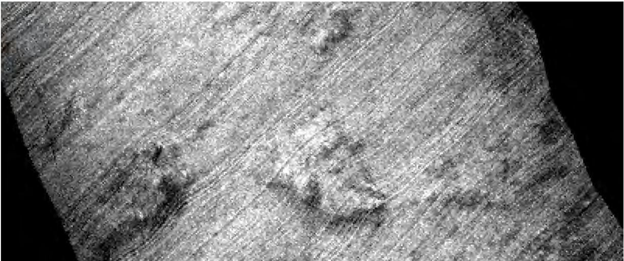
Figure 40. Zoom-in to a selected part of a UHI recording showing noisy spectral bands along and across-track.
