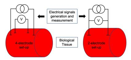
Figure 1. 4-point and 2-point bioimpedance measurement set-ups.
