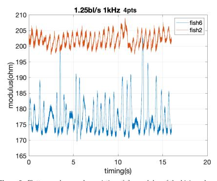
**Figure 5.** Plotter graph example: variation of the modulus of the bioimpedance over the 16s measurement for two fishes. The water speed is 1.25 bl/s, the bioimpedance measurement setup is 4 pts, and the bioimpedance frequency measurement is 1 kHz.
