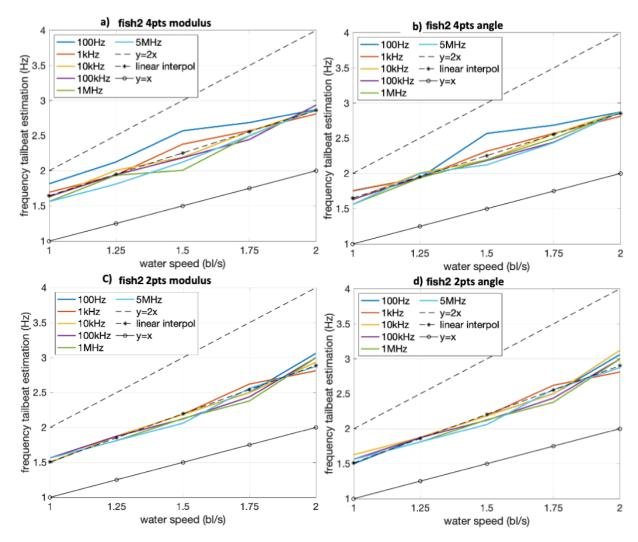
**Figure 6.** Water speed versus bioimpedance-based TBF estimation for fish 2 (a) 4 pts modulus of bioimpedance for frequency estimation; (b) 4 pts angle of bioimpedance for frequency estimation; (c) 2 pts modulus of bioimpedance for frequency estimation, (d) 2 pts angle of bioimpedance for frequency estimation.
