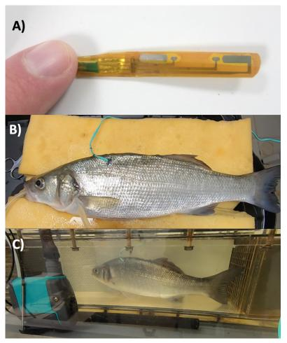
**Figure 2.** (**A**) The flexible biocompatible 4-contact electrode for bioimpedance measurement; (**B**) Fish after surgery for implantation of the electrode; (**C**) post-surgery fish recovery in the Steffensen-type swim tunnel.
