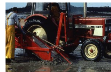
Harvesting Japanese carpet shell using a tractor equipped with a blade and conveyor belt (hard bottom)
