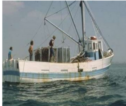
Oyster barge deploying iron frames for spat collecting and bag growing
