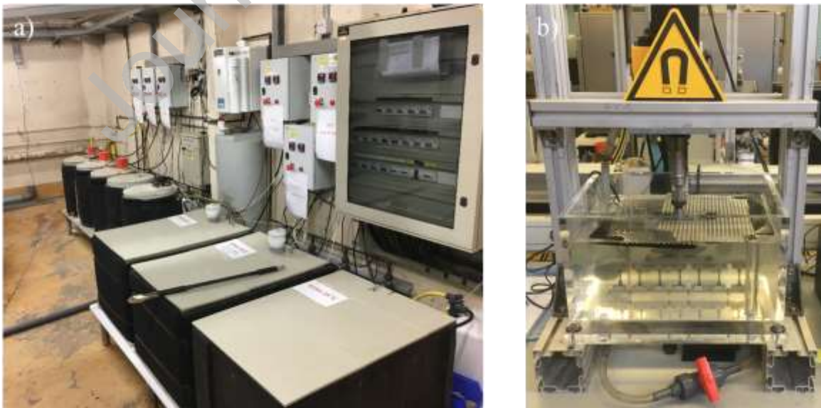
Figure 1 : a) Seawater tank facilities used to perform accelerated ageing. b) Custom fatigue experimental setup in seawater, adapted from [26].
