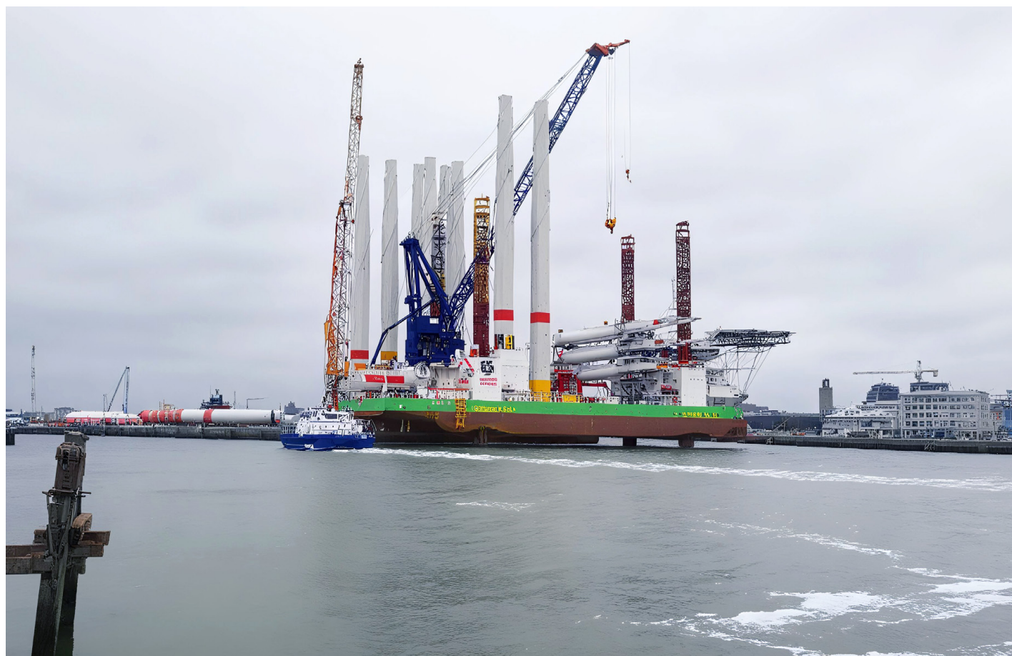
Wind turbine installation vessel being loaded in Ostend, Belgium
