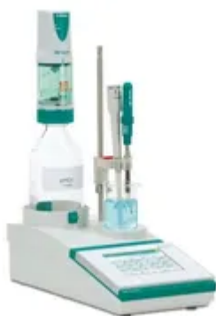
Figure 16: Metrohm Ti Touch 916 oxygen analyzer with a platinum titrode, a 20 ml burette to deliver the sodium thiosulfate and a 5ml burette to deliver the potassium iodate
