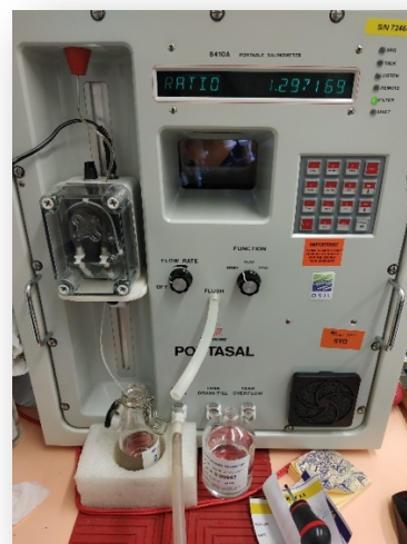
Figure 17: Guildline portasal 8410A salinometer
