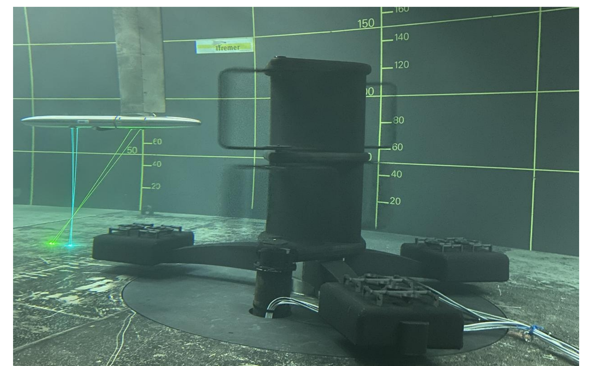
1/20 scale model of the HQ 2.5 in the wave and current flume tank for performance and flow characterization
