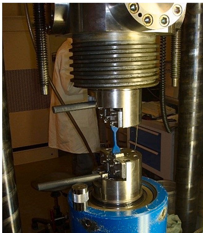
Fig. 8. Hyperbaric pressure chamber on mechanical test frame to study mechanical response under pressure, Cartié et al., 2006
