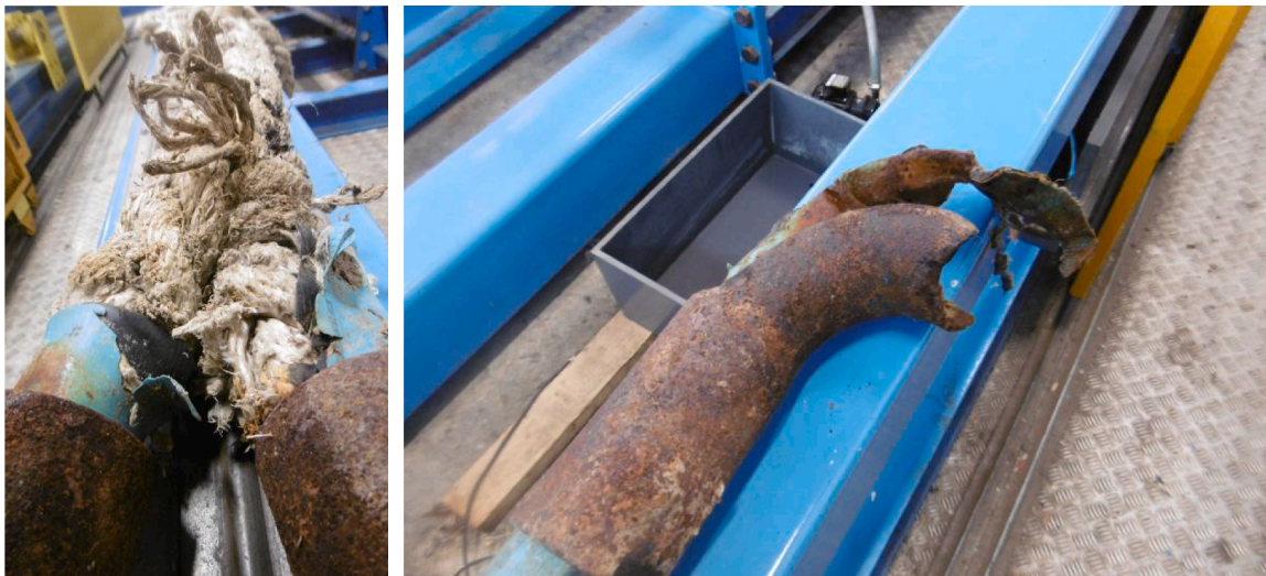
Fig. 17. Thimble contact causing damage to strands after protective cover failure (I-7) or corroded thimble failing during test (I-9).
