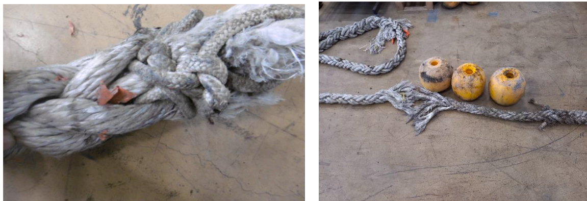
Fig. 10. Failure zones of ropes tested with floats.
