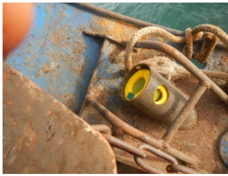
Figure 3: Ifremer NourDem trawl 11.90-16.45 m. Detail of the arms and braces (bottom left). NetSonde" sensor positioned at the center of the back rope to measure the trawl's vertical opening (top right). Panel gap sensor positioned on a panel (center right), and PC screen allowing live monitoring of panel gap and inclination/angulation throughout the tow (to validate the tow, or possibly cancel it if the gap falls outside the tolerances set at 15 and 20 m).
