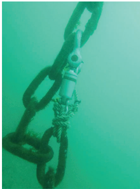
Figure 2: Load sensor set-up in one of the mooring lines ©Ifremer (2023).
