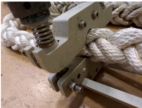
Fig. 11. Detail of clamping system.
