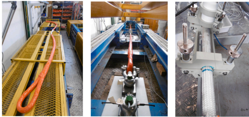
Fig. 24. Images of rope on laboratory test frame showing load sensor (middle) and wire transducer (right).
