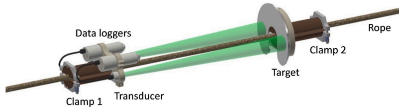
Fig. 2. 3D picture of the first acoustic strain sensor prototype.
