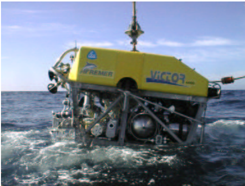
Figure 1: The Ifremer Victor 6000 underwater ROV (© Ifremer)
