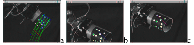
Figure 6: Effect of the pan/tilt control: the desired position of the object in the image is modified. (a) initial position, (b) desired position with no pan/tilt control, (c) desired position with pan/tilt control.
