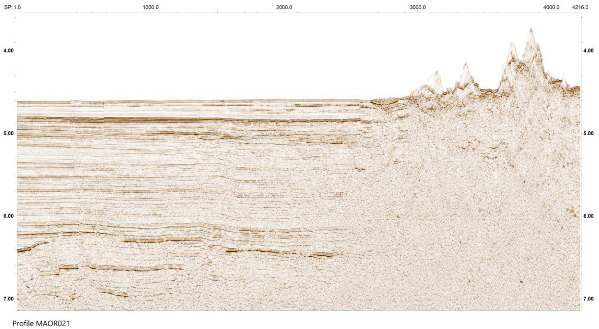
Figure S3-4: Uninterpreted seismic profile MAOR021. Legends and units as in Figure S3-2.
