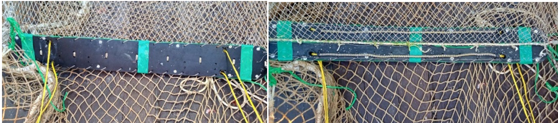
Figure 9.61. Full-scale kite (122 x 15 x 1.3 cm) in a trawl, front (left) and back (right) views. A steel coil tube on the back of the kite guides and protects the control lines.
