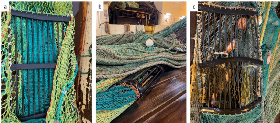
Figure 9.46. Pictures of a grid in the new flexigrid section (a), a grid in the used flexigrid section deformed on deck (b), and a grid in the used flexigrid section laying on deck (c).
