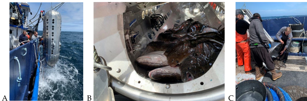
Figure 9.64. Shuttle being retrieved (A), catch entrained in shuttle (B), and catch being emptied onto the vessel deck (C).
