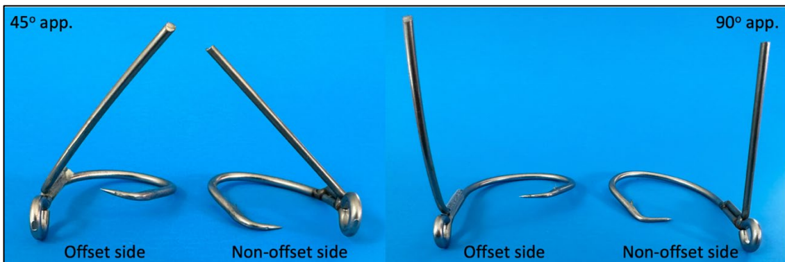
Figure 9.70. Images comparing 45o and 90o appendages (app.) extending outwards from the hooks shank on the hooks offset and non-offset side.
