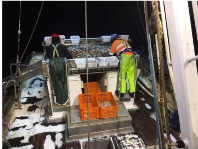
Figure 9.3. Traditional sorting of the catch. Crew manually separate prawns from the catch before disposing of bycatch overboard via a chute.
