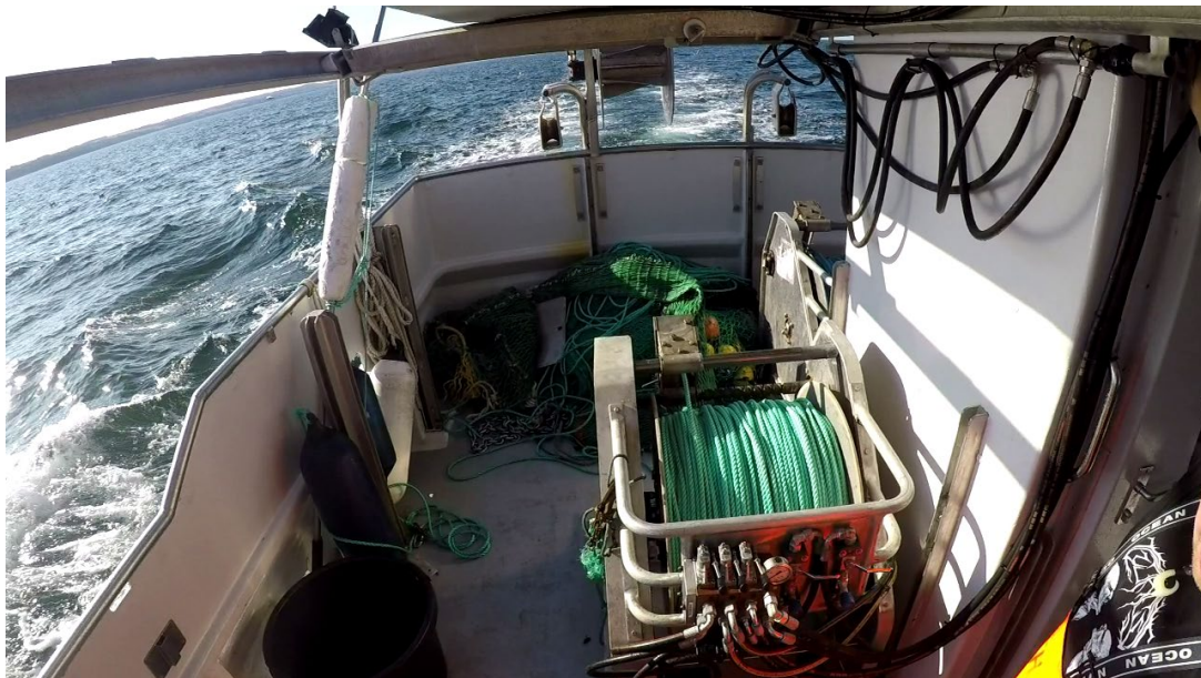
Figure 9.28. Mini seine system installed onboard the Danish fishing vessel being involved in previous work with it.
