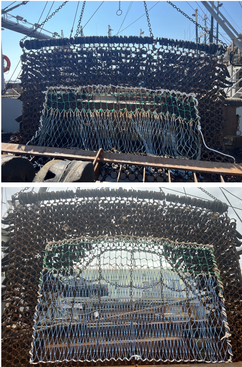
Figure 9.71. Images of the seven-row apron dredge with the two-row square mesh escape panel (top) and three-row square mesh escape panel (bottom).
