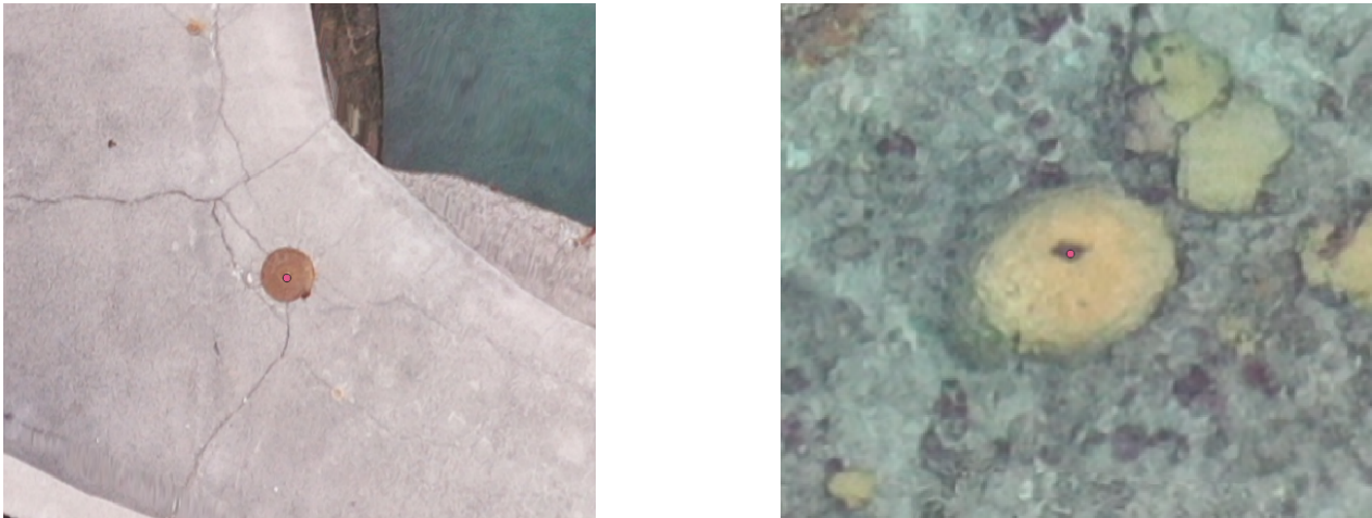
Figure 12: Examples of Ground Control Points (GCPs) collected in Reunion island in order to correct the aerial orthophoto position. Both human made objects (on the left) and easily distinguishable corals (a Porites coral on the right) can be used to set GCPs.
