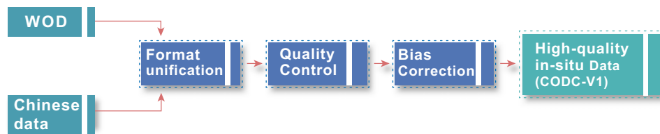
Fig. 3 Flowchart illustrating the main workflow, data source, and techniques used in CODC-v1.
