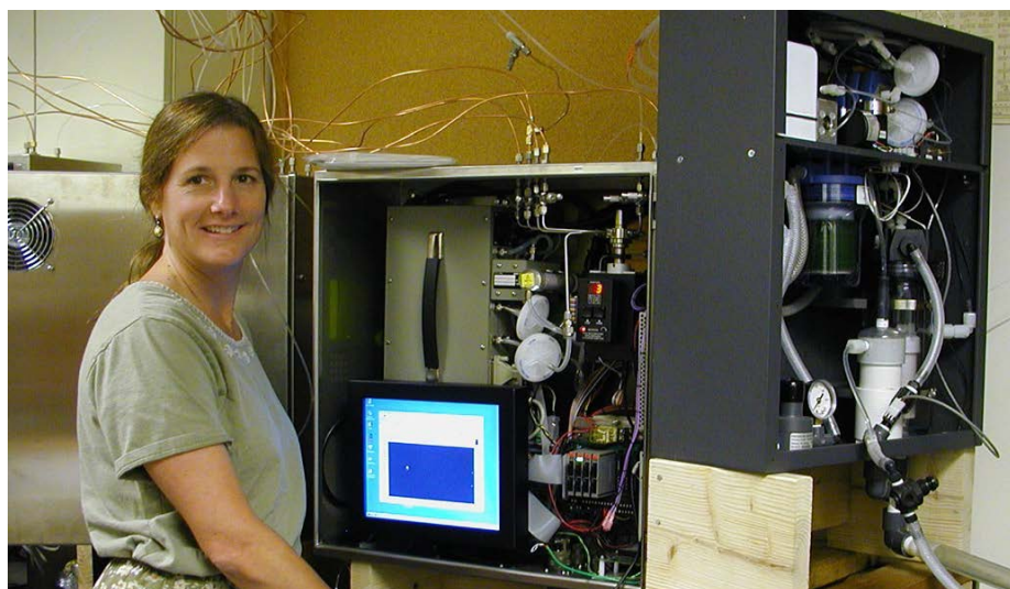
FIGURE 2. The NOAA Pacific Marine Environmental Laboratory (PMEL) underway f\text{CO}_2 system, originally designed by Craig Neill, is a two-box measuring system (“dry box” at left, “wet box” at right), being maintained here by Cathy Cosca of PMEL.
