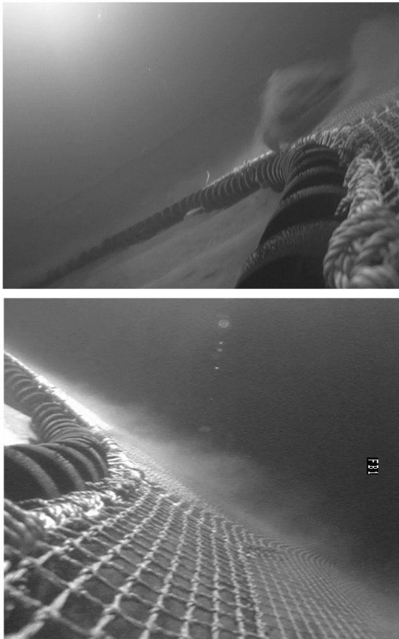
Figure 4.11. Light hopper ground gear, showing centre round to the starboard wing (top) and the quarter/belly guard meshes (bottom).
