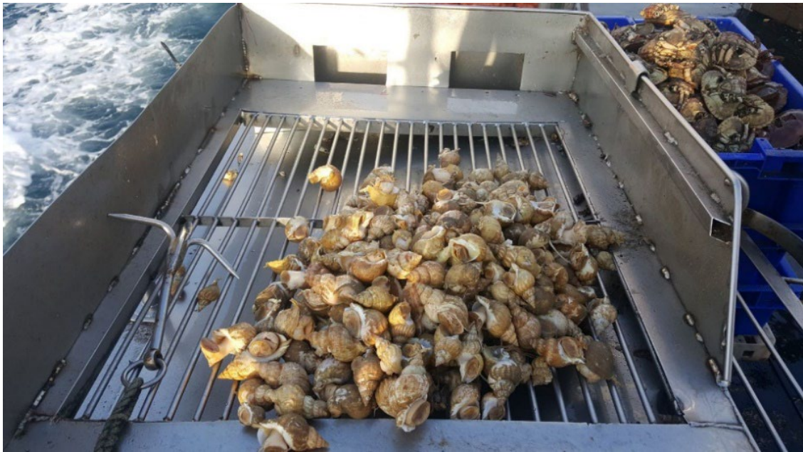
Figure 4.18 Whelk riddle used to separate whelk above the size of set bar-width from smaller individuals under minimum landing size (image copyright: Jack Emmerson).
