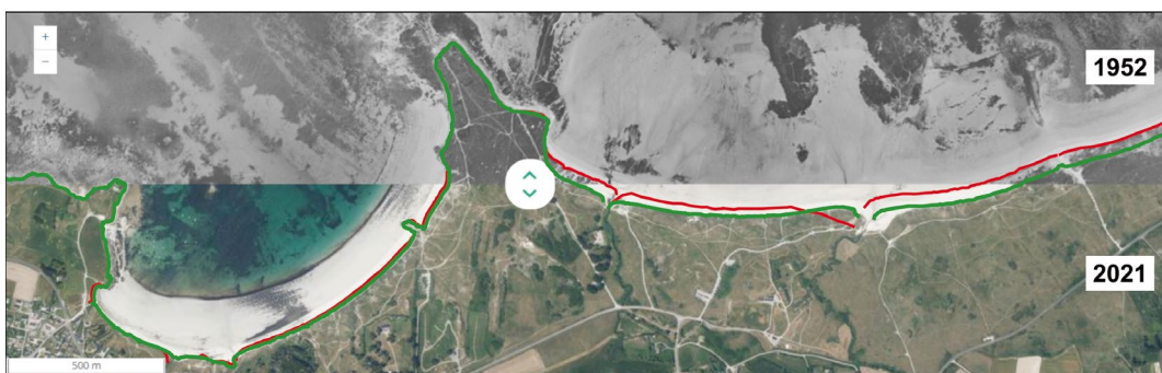
Fig. 10.1 Coastline recession visible by comparing two aerial images from 1952 (coastline digitized in red) and 2021 (coastline digitized in green). Location:
