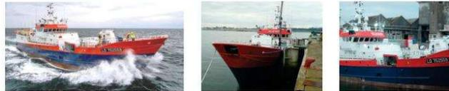
Heliotrope is the name of the longliner. It is a former trawler of 33.8m. Autoline system makes it possible to deploy about 30 km of lines and 25000 hooks each 24 h. Crew is made of 13 sailors. First time his technic is tested in France.
