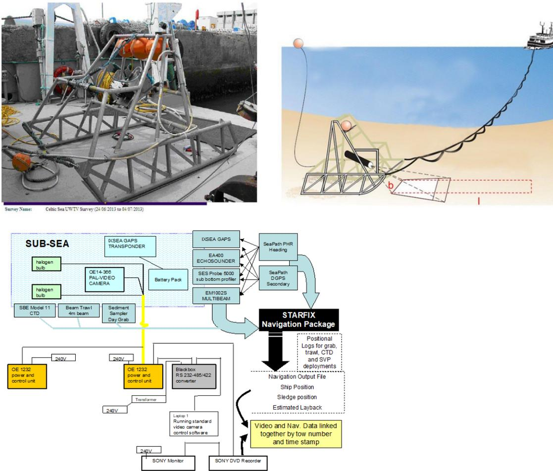
Figure 4. Schematic diagram of the sledge and traction on the sea bottom. Mechanism for acquiring process onboard. Source: Marine Institute, Ireland.
