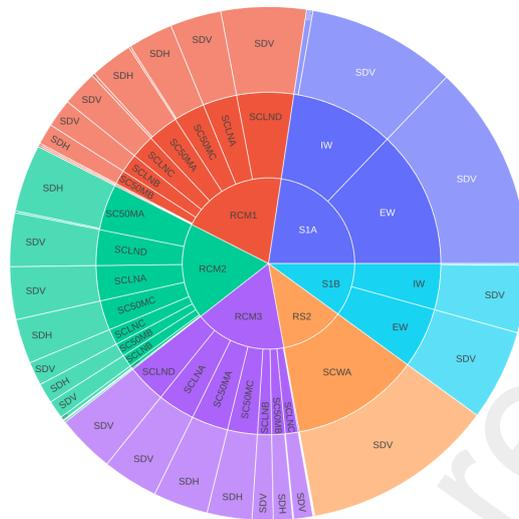
**Fig. 3.** SAR constellation contributing to the TC monitoring with sensor names (inner circle), acquisition modes (middle circle. Refer to missions product format description for details of each mode) and polarization configurations (outer circle. SDV means VV and VH, SDH means HH and HV, SSH means HH and SSV means VV) available.
