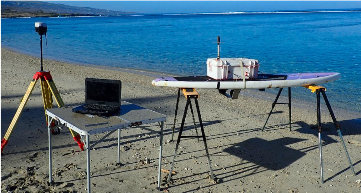
(a) ASV preparation for a survey operating remotely with the mobile GPS RTK base station (on the yellow tripod)
