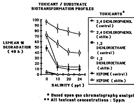
Figure 2 : Toxicant/substrate profiles for 2,4 DPH, 1,2 DCE, and KP.
