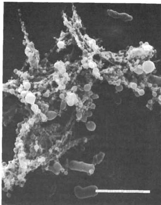
Figure 4 : Scanning electron micrograph of colonized chitin in the presence of 1,2 DCE.
