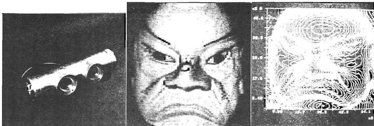
Fig. 5.1 Spotscan-3D. a) Subsea instrument housing. b) Radiometric image. c) Contoured plot
