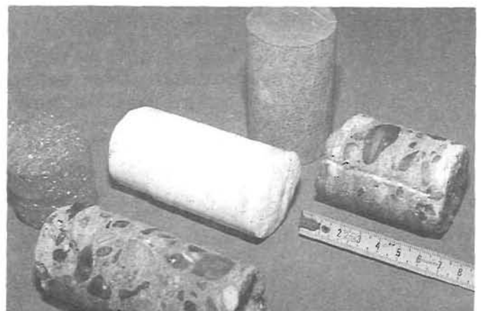
Fig. 4 : Test Cores of various Materials : Concrete, Brick, Marbel and Basalt
