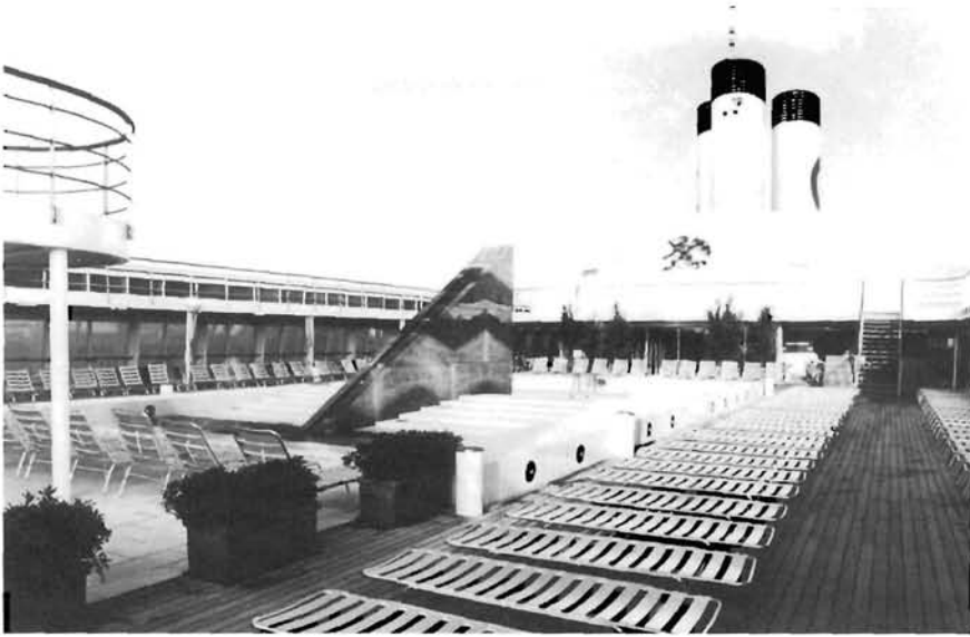
1 - Paquebot "Costa Classica" - Cheminées FRP Cruise passenger vessel "Costa Classica", FRP funnels.
