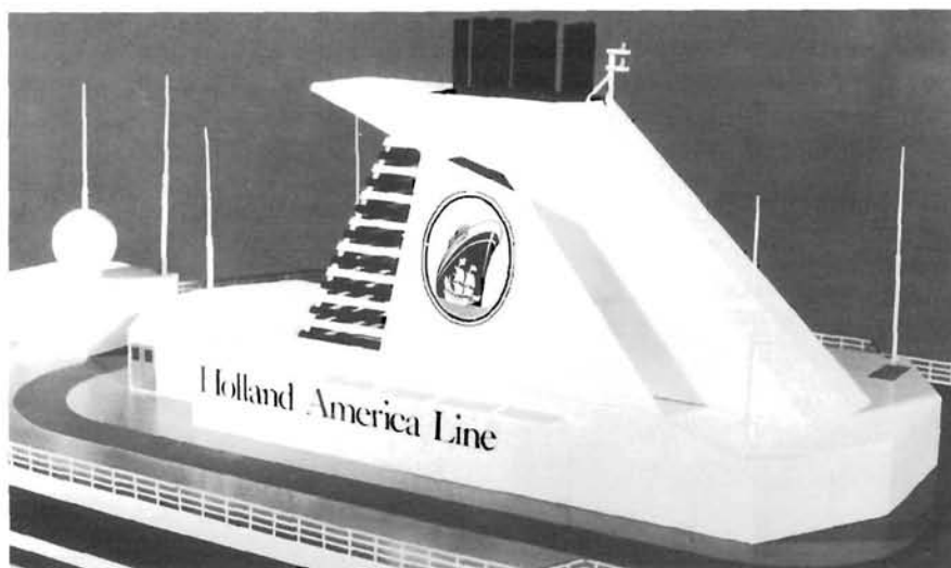
3 - Paquebot "Statendam" - Cheminée FRP Cruise passenger vessel "Statendam", FRP funnel.
