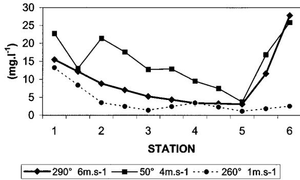
Figure 7. Wind effects on the SPM concentration. Values are depth averaged.
