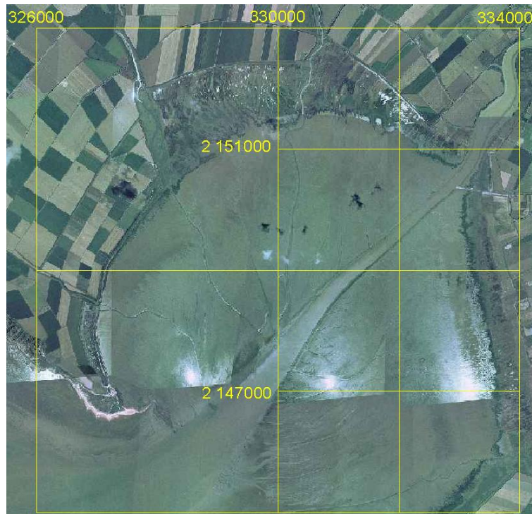
Figure 4: Orthophotograph of Aiguillon cove (August 2, 2000) and extensions of photogrammetric DTM calculations. Coordinates are in the metric Lambert system.
