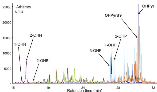
**Fig. 2.** GC/MS chromatogram (SIM mode) as an example of bile analysis for PAH metabolite determination. (OHN = hydroxynaphthalene, OHBi = hydroxy-biphenyl, OHP = hydroxyphenanthrene, OHPyr = hydroxy-pyrene)
