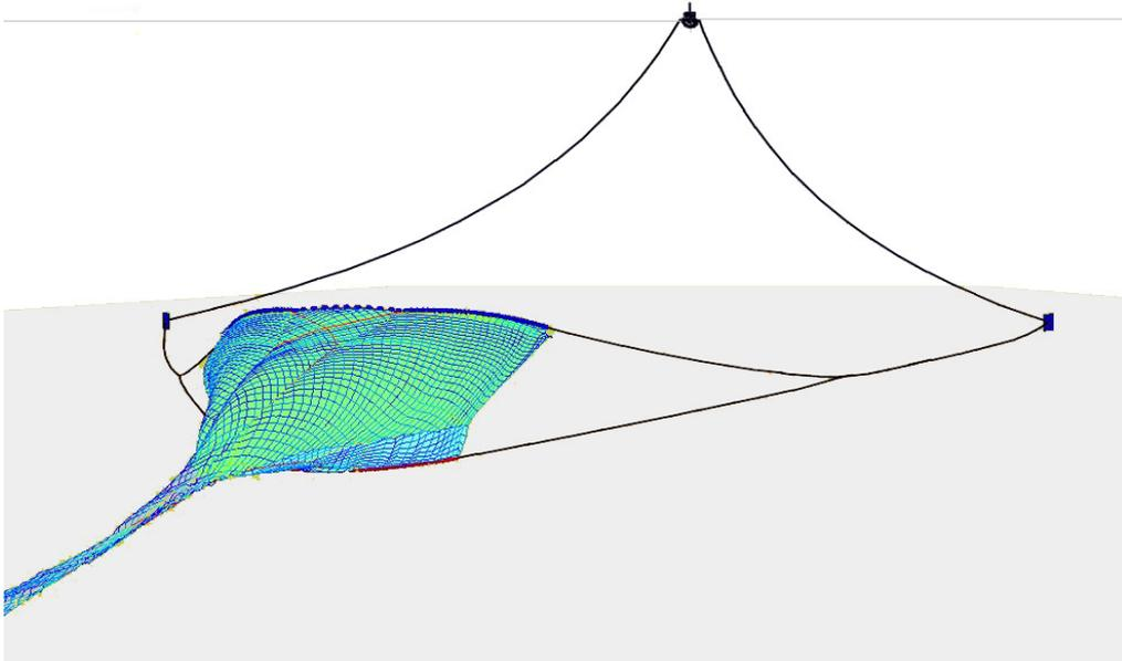
Figure 7. Numerical simulation of the equilibrium of the complete trawl gear
