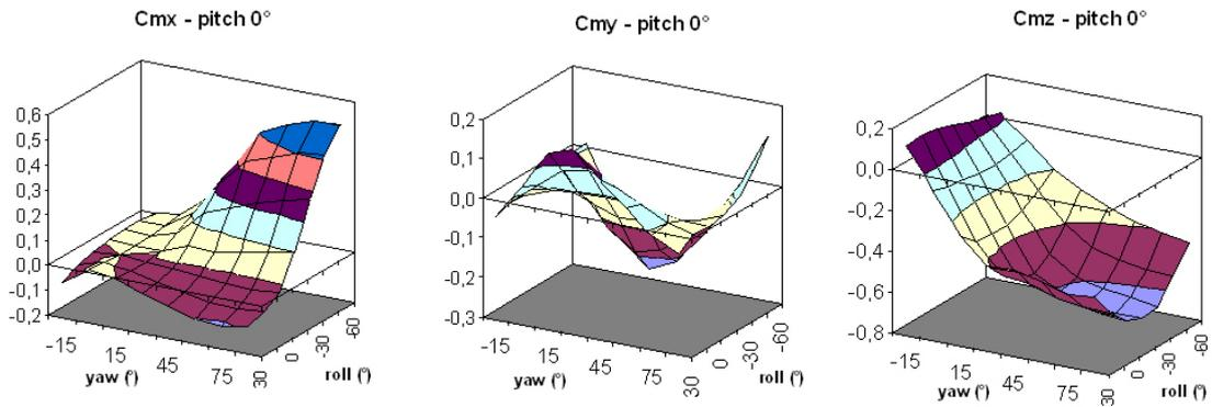
Figure 5. Variations of the door coefficients with yaw and roll (pitch = 0°)
