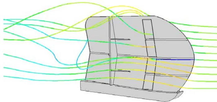
Figure 4. Path lines around the trawl door (yaw 15°, pitch 0°, roll 15°)
