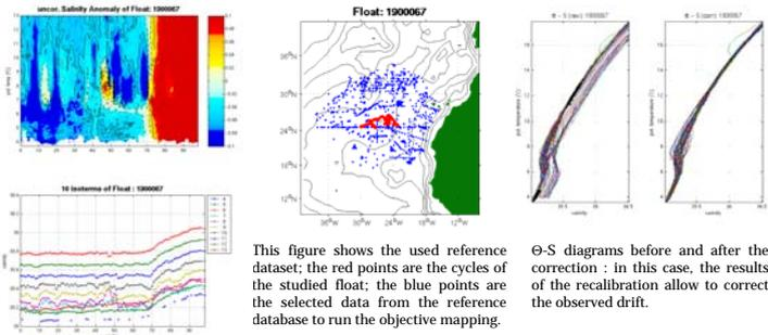
This figure shows the used reference dataset; the red points are the cycles of the studied float; the blue points are the selected data from the reference database to run the objective mapping.
